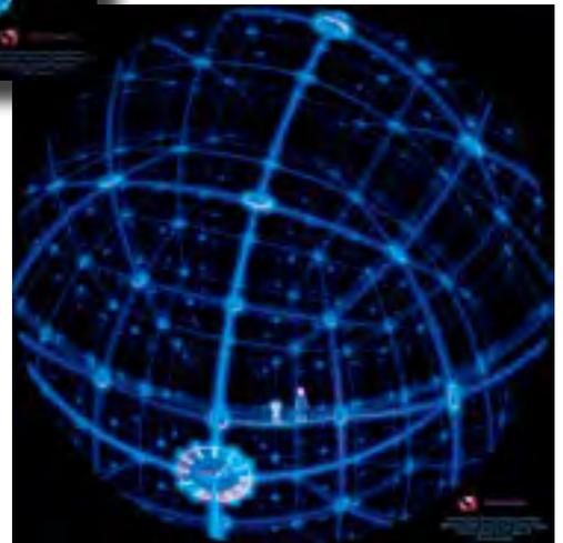
system, a constellation of satellites that tell navigation systems where they are exactly. GPS depends on the precise measurement of time. Every one of the 24 active satellites simply broadcasts its own time. By measuring the time differences between the signals of the satellites, the navigational system can determine its own location on Earth.
